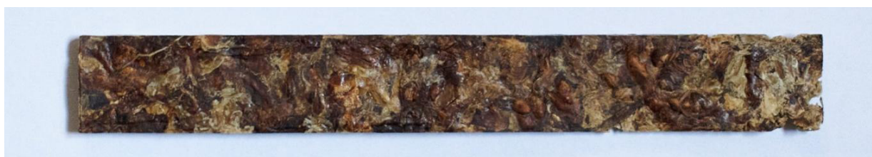
Fig. 1 – A sample of briquetted alternative solid fuel from the dried beet pulp.
